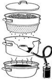
The units are generally made in a three-tier configuration that resembles a huge double boiler.
